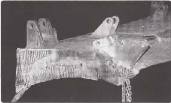
Dozer Blade hardfacing with LoTherme-604
