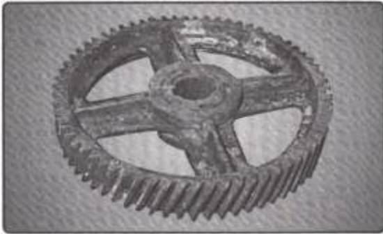
Cast iron gear repaired with LoTherme-703
