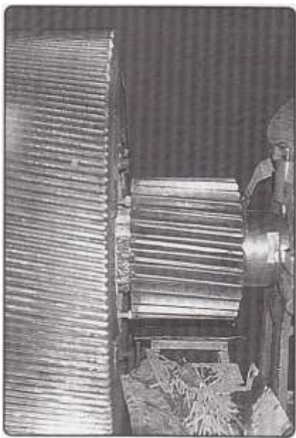
Gear Teeth built up with LoTherme-601
